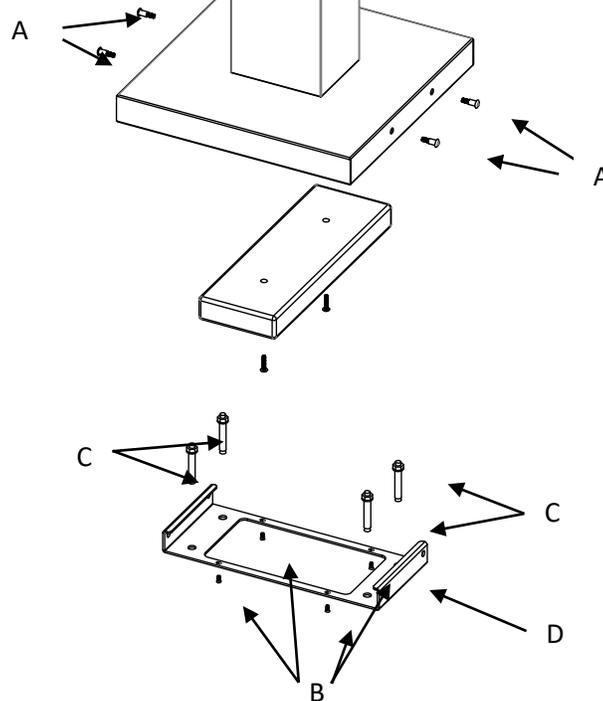
**Important Notice:** The anchors (C) shown in the above diagram are not included with the pedestal base and must be supplied by the installer/owner.
